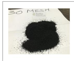
Continued processing with a granulator or cracker mill, possibly with the aid mechanical means, reduces the size of the particles further.
