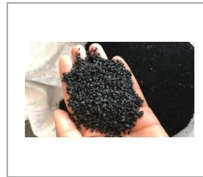
**Crumb rubber** is recycled rubber produced from automotive and truck scrap tires. During the recycling process, steel and tire cord (fluff) are removed, leaving tire rubber with a granular consistency.
